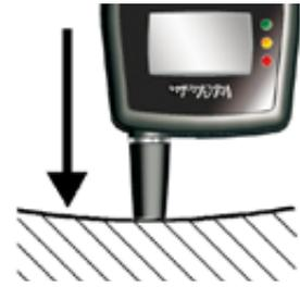
Rubber sleeve in contact with the surface. Hold steady.
