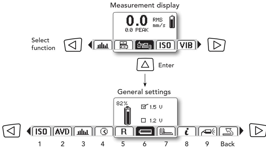
The lower part of the **Measurement** display contains five function icons. Use LEFT/RIGHT arrow buttons to highlight the **General settings** icon, then press the UP arrow button to enter.
