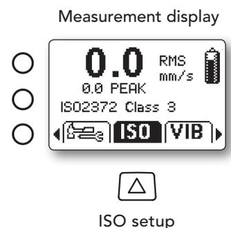
When ISO 2372 is activated in the **General settings** display, the machine CLASS (1-6) is selected in the **ISO setup** display with the UP/DOWN arrow buttons. Save and return with LEFT arrow button.
