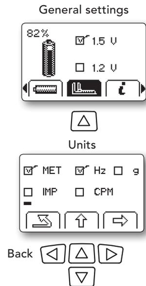
Setting of units will affect the date format. With the MET (Metric) setting, the date format is YY-MM-DD. With the IMP setting, it is DD-MM-YY.
