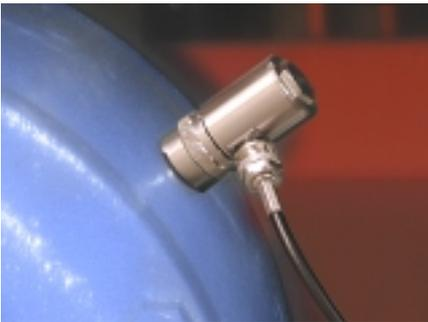
Special transducers for shock pulses and vibration assure accurate measurements. On measuring points that are inaccessible during normal operation, the transducers are permanently installed and connected to measuring terminals.
