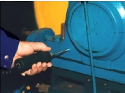
Speed data are necessary for condition evaluation, and monitoring the machine temperature often supplies valuable information. T30 uses temperature probes for solids and liquids. Speed is measured by contact, or optically from a safe distance.
