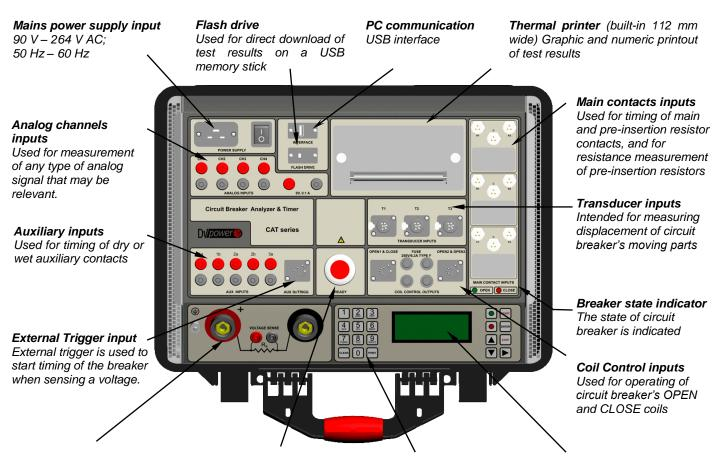
*Micro Ohmmeter* (built-in 500 A DC micro ohmmeter) for static and dynamic contact resistance measurement
