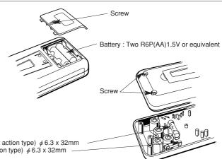
Fuse: F 600V/10A (Fast action type)  $\phi$  6.3 x 32mm F 600V/800mA (Fast action type)  $\phi$  6.3 x 32mm
