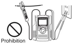
♦ Hold the test leads in the holster, while making the frequency measurement by using the clamp sensor. Hold the clamp sensor in the holster, while making the frequency measurement by using the test leads.
