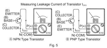
(7) The leakage current of the silicon transistor is too small to give pointer deflection. If the pointer should deflect, the likely cause would be some fault of the silicon transistor.
