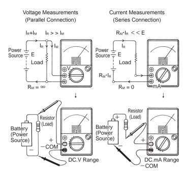
Measuring voltage at both ends of a resistor.
