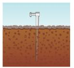
Earth measurements are possible up to 100kΩ\* of auxiliary earth spikes resistance.
