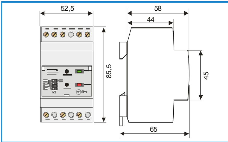
Snap on DIN rail 35mm
