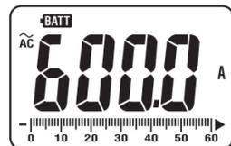
Replace the batteries when a Low Battery Voltage warning "BATT" mark is indicated on the display. Note that when the battery is completely exhausted, the display blanks without "BATT" mark shown.
