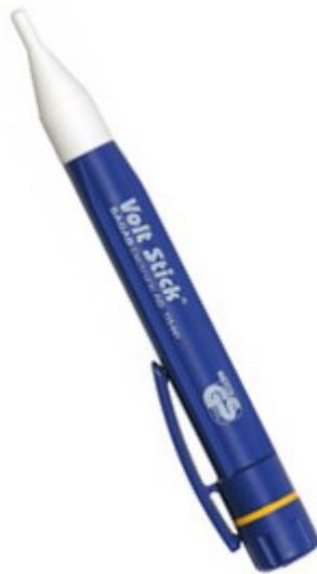
The Volt Stick is an instrument for safely checking for the presence of an AC voltage in cables, wall sockets, fuses, junction boxes, etc. No current flow is needed for correct operation. Voltage indication by means of a bright light signal in the tip. Examples of applications areas:
